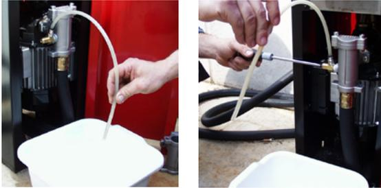
2 Put the small pipe connected with the RELEASE VALVE in a vessel and open the valve with a screwdriver.
