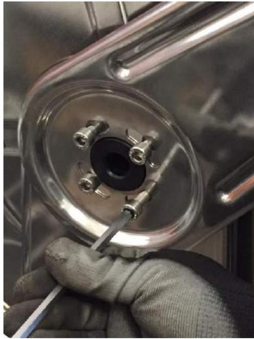
Take out the 4 screws with proper allen key
