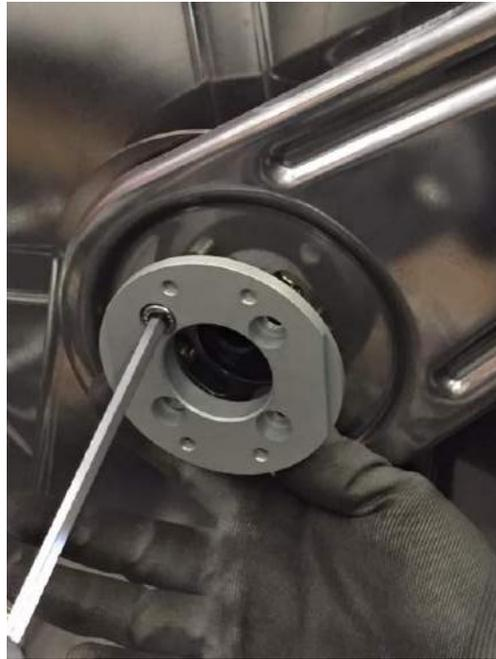
Fix the adapter with the 4 screws just dismantled
