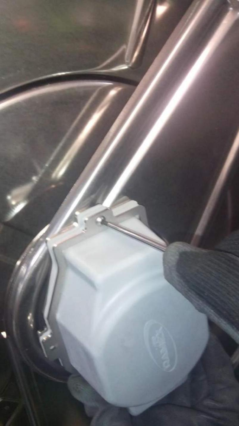
Fix the external frame adapter then tighten the four screws.
