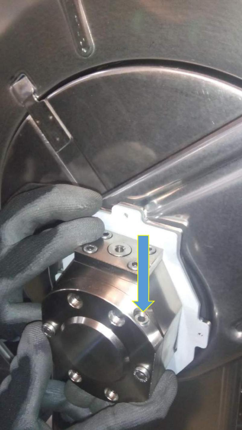
Put the brake on connection shaft.
