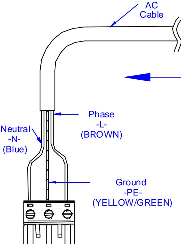
Remove the connector from the package and insert the power cable as shown in figure
