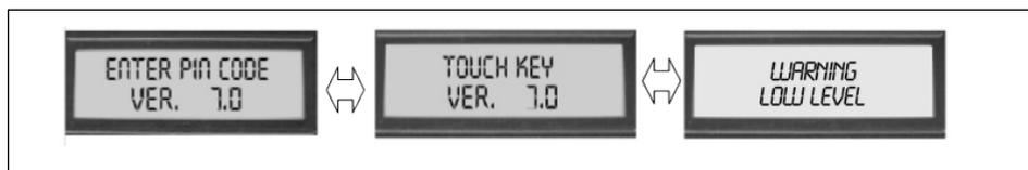
These messages display when AGILIS is waiting for a PIN CODE or for a KEY to be touched to the reader, or when there is an active level alarm.
