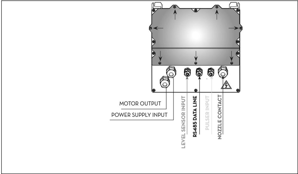
Once the cover has been opened, the electronic board and its connectors are accessible:
