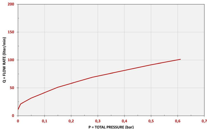
**TIPO DI FLUIDO** DIESEL**TEMPERATURA** 14,8 °C**DIMENSIONI**
