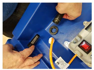
2. Unscrew the grey cable gland to free up the orange electricity cable from the tank. Remove the other side of the cable from the switch located in the battery holder (4 screws to remove the battery holder), pass cable throught the cable cable into the
