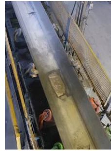
Crack repair in copper mine Steel cord belt rip
