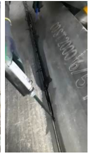
Crack repair in copper mine Steel cord belt rip
