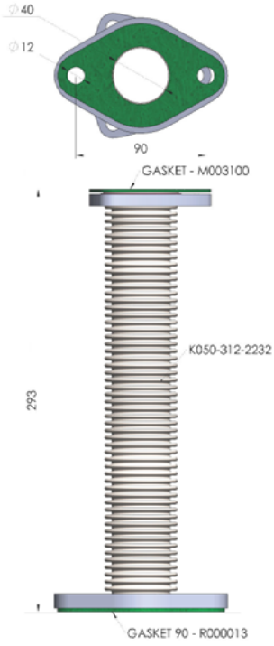
TW connecting hose DN40 - 90 mm - 290 mm
